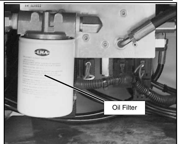
Figure 3-14: Hydraulic Oil Filter from left side
