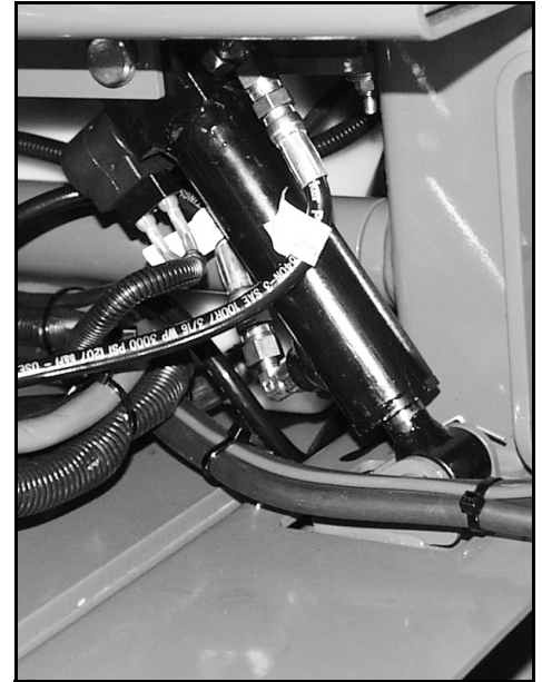
Figure 3-23: Depression Mechanism Cylinder
